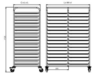
Carro self service tubo Ø 25 | Trolley self service tube Ø 25 | Chariot de service tube Ø 25
